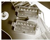
While the overall tone and dynamic character of Ellis' LRP and Betty sets clearly share the same DNA, the Betty pickups sound slightly less compressed and brighter in the style of a P90, while still retaining the fuller
